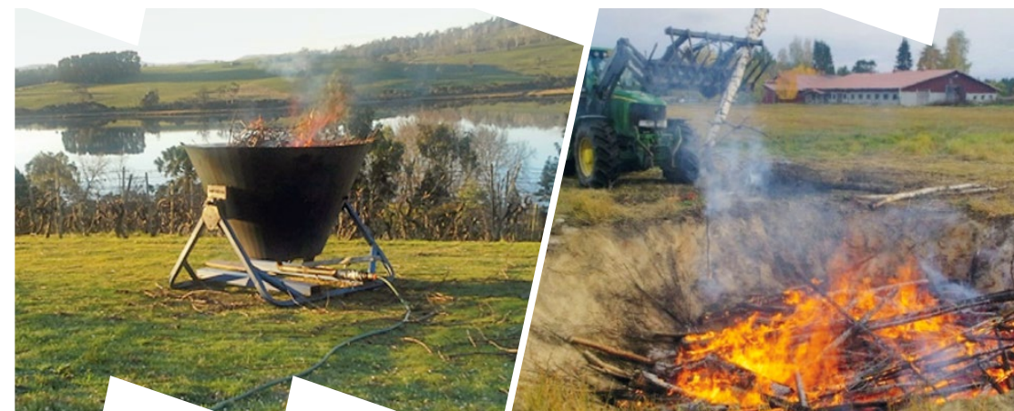
Figure 3. left: Kon-Tiki kiln in Tasmania by Frank Strie, one of the first models for activating the hot biochar by bottom-up quenching with water. Photo from [20] . Right: Large-scale pyrolysis in soil pit is an efficient way of getting biochar on farm- it is though crucial to have good set of long tools to arrange biomass in even layers to avoid smoke emissions. It is also recommended to have the walls of soil pit covered by clay plaster to facilitate easier collection of liquid-activated biochar after quenching. Farm-scale pyrolysis event in Liperi, Finland in October 2019. Photo by Priit Tammeorg
