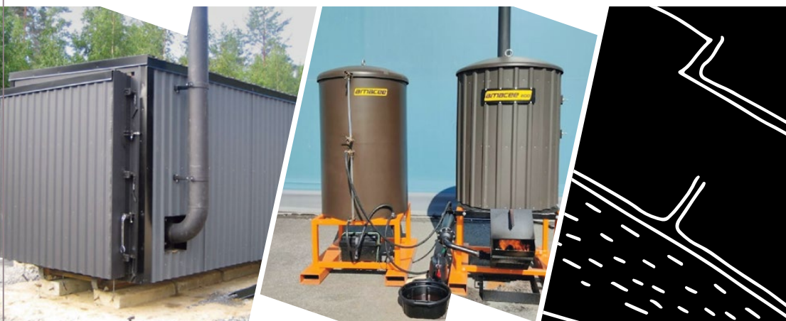
Figure 2. Two types of batch retorts suitable for decentralized biochar production. Photos by Tuomo Leppänen
